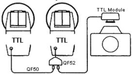
Accessories needed: One Control Cable QF50, one "Y" Module QF52, and one TTL Adaptor.
