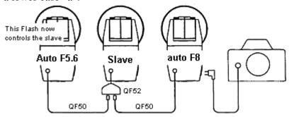
Accessories needed: Two Control Cables QF50, one "Y" Module QF52 and one sync cord.
