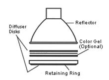
There are also two options (sold separately) for adding color gels. QF65 Clear UV Filter Kit, can hold color gels to provide non-diffusing color. QF66 Color Gel Set, contains 7 pre-cut gels that fit QF64 or QF65.
