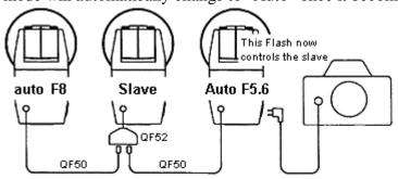
Accessories needed: Two Control Cables QF50, one "Y" Module QF52 and one sync cord.
