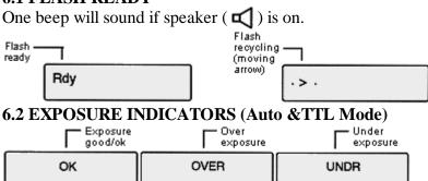
The exposure indicators will come on and blink for approximately 3 seconds after a flash. If the speaker is turned on then a warning will sound three beeps if the exposure is Under or Over. If the exposure is good, one beep will sound when the flash is ready, and the OK will display.
